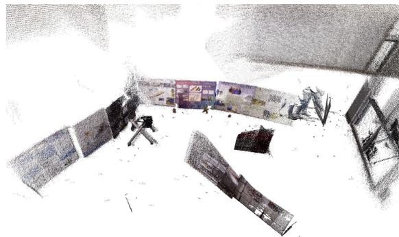
Figure 4. Generated 3D map of the indoor environment we made. Some posters we used as wall, the bumblebee action figure, water bottle, chair, and windows are visible in the generated point cloud.
