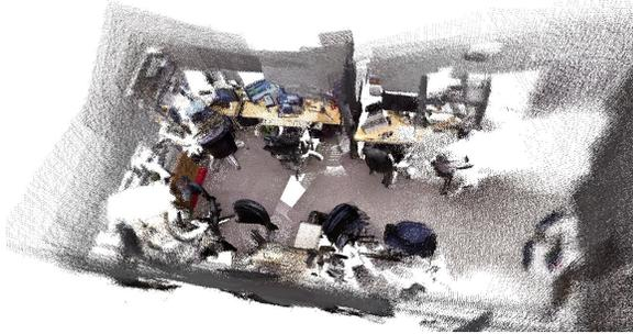
Figure 5. 3D map of our office generated by graph-based SLAM algorithm.
