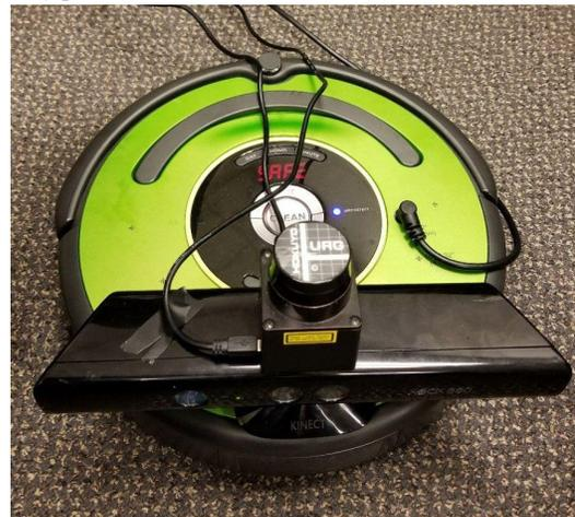
Figure 1. Robot and vision setup
